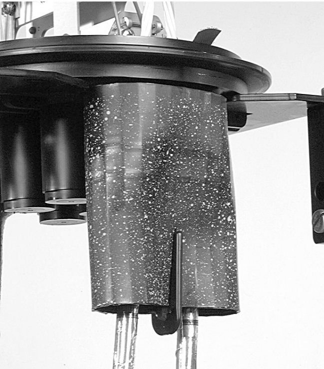
5.1.5 Push the sleeve against the base and place the clip.
