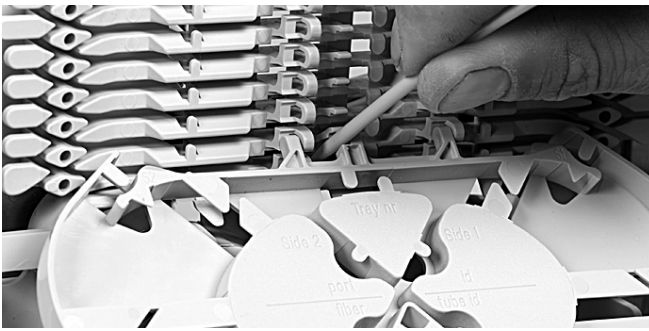
6.5 To remove the tray put the fiber guiding pin between lip on wraparound groove plate and tray and move lateral towards S1.
